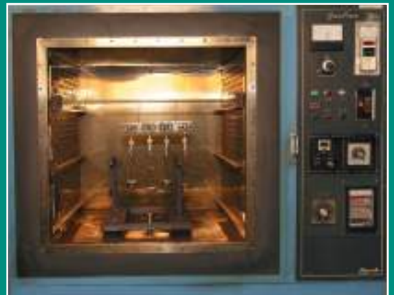
XLPE Hot Set Test Equipment - Oven
