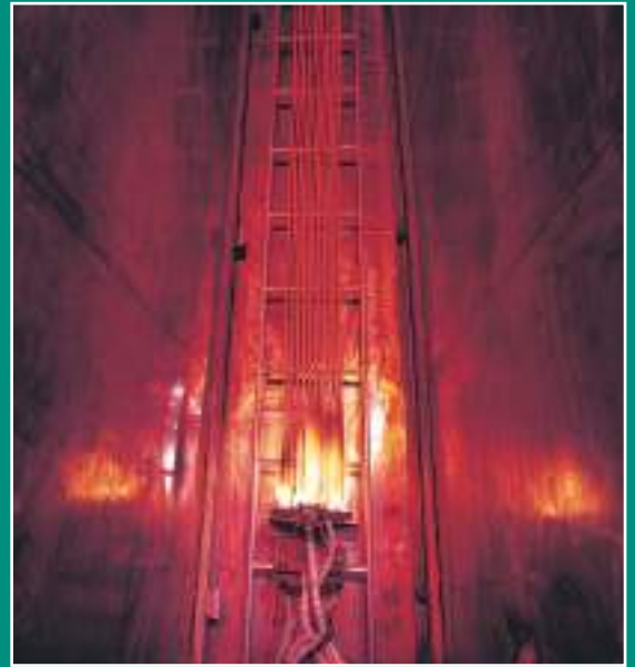
Flame Retardant Test Equipment - IEC 60332-3
