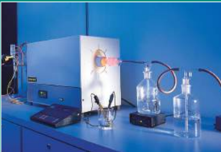
Halogen Content & Corrosivity Tests Equipment - IEC 60754-1 & IEC 60754-2
